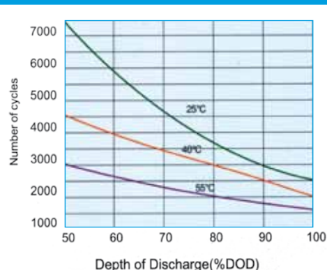
Cycle life versus DOD and temperature at 0.2C
